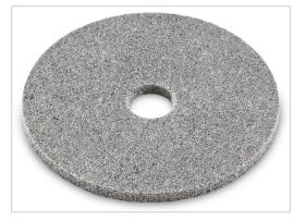
For grinding welds and removing tarnish. High-quality surfaces at welded joints in a single work step. The perfect disc for quick and high-quality fillet weld processing. Ideal for alloyed and high-alloyed steels, chromed and nickel steels, titanium, light metals, non-ferrous metals and steels. Pre-grind weld under 6A medium, 3S fine for finishing.
