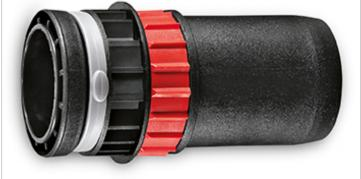
For connecting a FLEX power tool to extraction units from other manufacturers. Suitable for hoses inside Ø 27 mm, outside Ø 36 mm, with auxiliary air adjustment.
